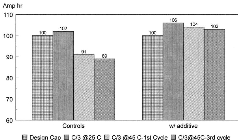
Fig. 3. The effect of metal hydroxide additive on the high-temperature charging efficiency. C/3 discharge capacities at 45°C during first and third cycles, compared with the designed capacity and that measured at 25°C.
