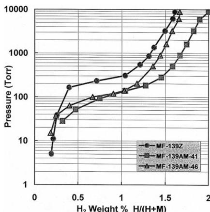
Fig. 4. Pressure-composition isotherm for standard (MF-139Z) and advanced hydride alloys.
